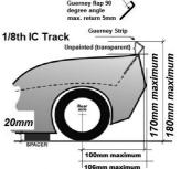
The maximum overhang is 100 mm measured from the rear axle centre point. See drawing.
